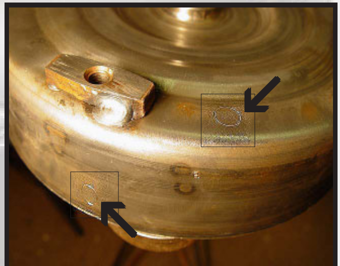
Figure # 2 Depicts 2 Degree Offset Mounting Pads
